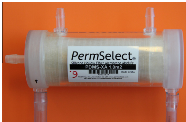
Fig. 1. The passive dosing unit showing the inlet (lower left) and outlet (lower right) ports for the perfusion of the lumen. The other three ports are for the perfusion of the shell space.
