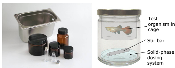
Figure 3: Actual passive dosing systems (left) and a conceptual CBR setup with guppy (right).
